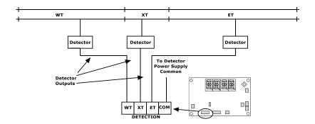
If storage tracks are present at your crossing, create XT track circuits for each storage track and include the circuits as the mainline XT. Any occupancy will show as the mainline XT. Additionally, optical sensors may be used in addition to current detectors on the XT to help ensure proper detection of trains.
