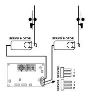
Install each servo directly under the respective gate signal so that a connecting rod can be aligned from the gate arm to the servo-motor output shaft lever. The CR-2 will by default place the servo motors in their middle position until adjusted. My powering the CR-2, the servos will assume their middle position. Then attach the gate arm to the servo at the 45-degree position. This will ensure a full range of motion for the gate movement.
