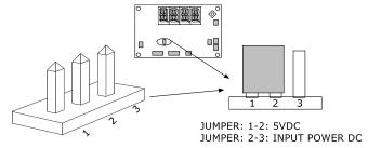
**NOTE:** JUMPER MUST BE SET TO PINS 2-3 WHEN USING THE CR-IR2 add-on board.
