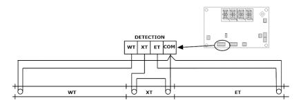
If storage tracks are present at your crossing, the XT is the only detection required for those tracks. This allows cars to be stored next to the road without operating the crossing. Additional MT-2 modules are not required. Simply include photocells for each storage track into the XT photocell string of the CR-2. Any occupancy of the storage track(s) will appear at the main track XT.
